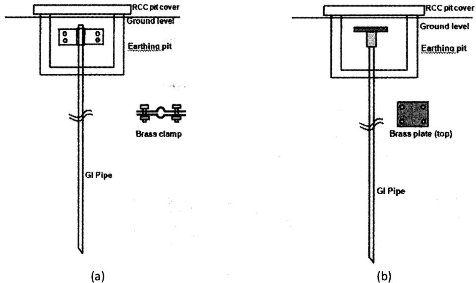
Figure 3 Pipe Earthing; (a) Type 1; (b) Type 2
