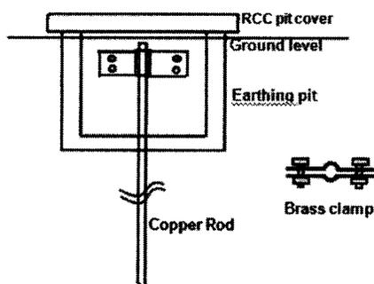
Figure 1 Copper Rod Earthing
